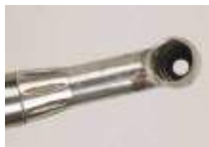
Figure 9. Corrosive effects of sterilization
