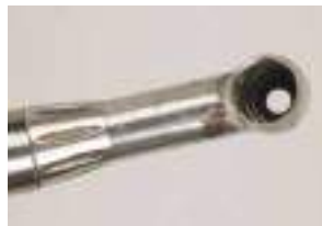
Figure 9. Corrosive effects of sterilization
